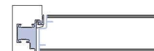
Ribasso (da 1 a 4 mm) - entrambi i lati / Both side lowered (from 1 to 4 mm)
